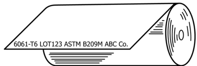
Fig. 1 Spot Marking for Coiled Sheet
