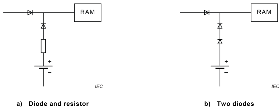
Figure 7 – Examples of wiring for charge protection
