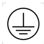
Figure 3 – Symbol for protective earth (protective ground)
