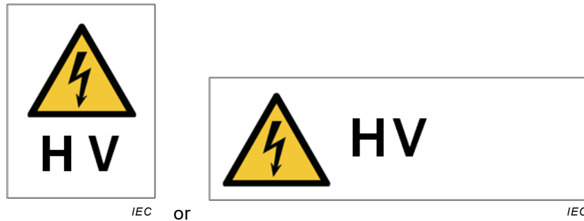
Figure 4 – Warning sign “high voltage”
