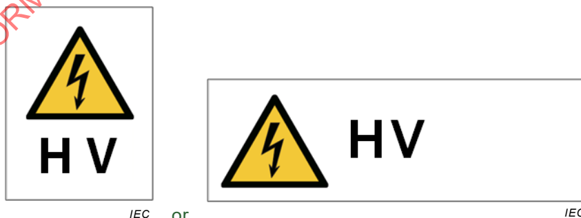
Figure 4 – Warning sign “high voltage”
