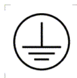
Figure 3 – Symbol for protective earth (protective ground)
