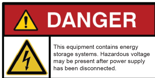
Figure 25 – Warning sign: energy storage system
