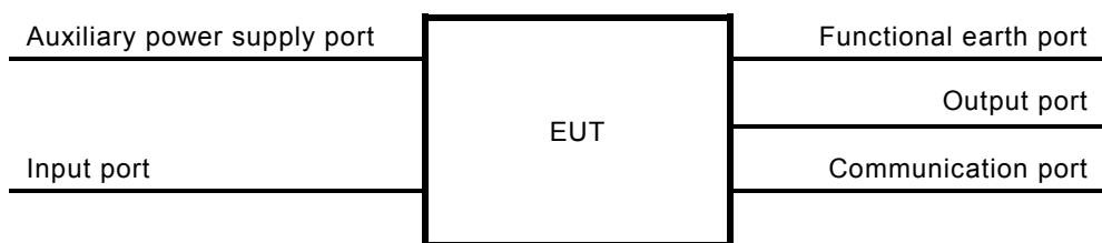
Figure 1 – Ports tested in this standard for measuring relays and protection equipment
