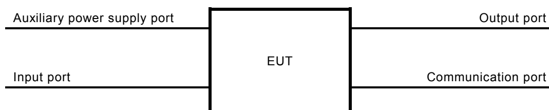
Figure 1 – Ports tested in this standard for measuring relays and protection equipment
