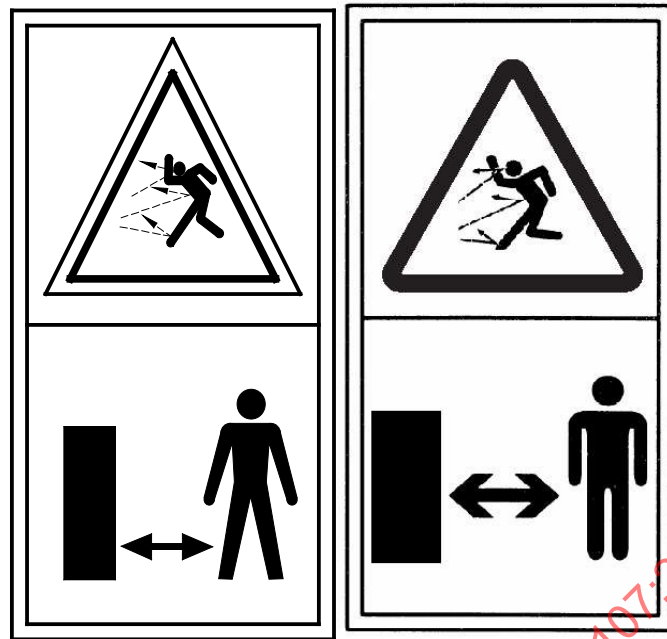
Figure EE.4 – Safety signs illustrating – "WARNING – Keep a safe distance from the machine when operating"
