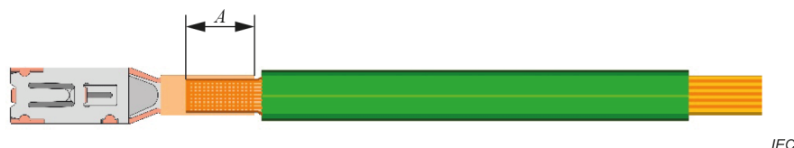
Figure 31 – Type D specimen at the wire to terminal connection
