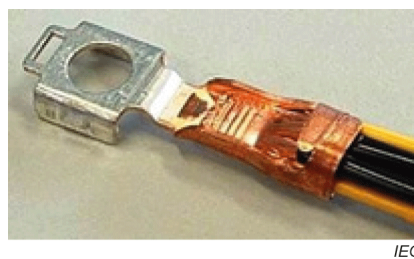
Figure 16 – Example of multiple wires welded to one terminal
