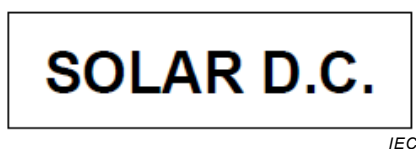
Figure C.712.1 – Example of sign required on PV array combiner boxes (712.514.102)
