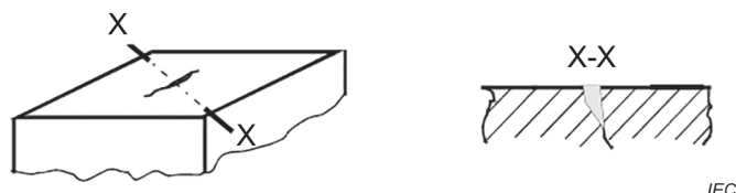
Figure 11 – Single-surface broad crack
