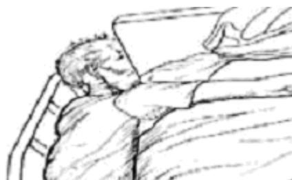
Figure AA.15 – Example of potential PATIENT entrapment in area C between SIDE RAIL and HEAD BOARD
