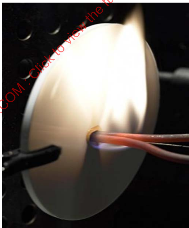
Figure B.1 – Example of a brightly shining flame
