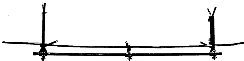
Porte-bretelle antivibratoire – Antivibration jumper installation tool
