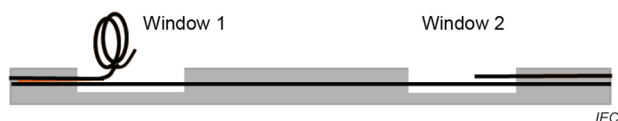
Figure 37 – Concept of straight midspan access
