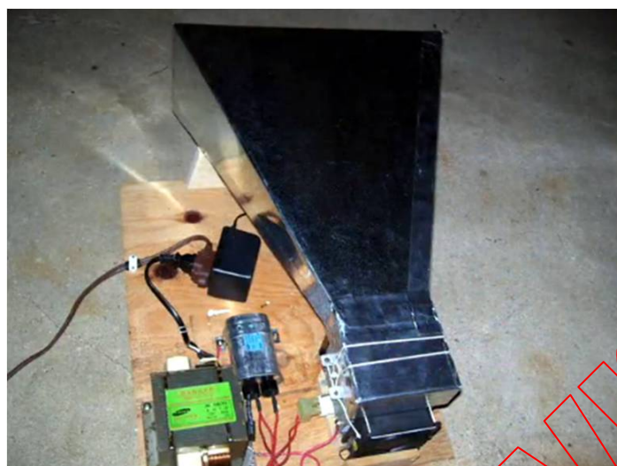
Figure B.9 – A do-it-yourself electromagnetic weapon made from an oven magnetron [13]
