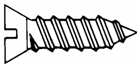
Figure 1 – Thread-forming tapping screw (3.6.10)
