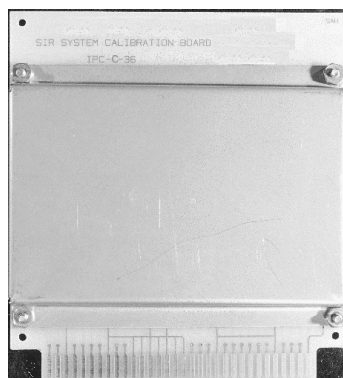
Figure 6 – Resistor verification board with protective cover
