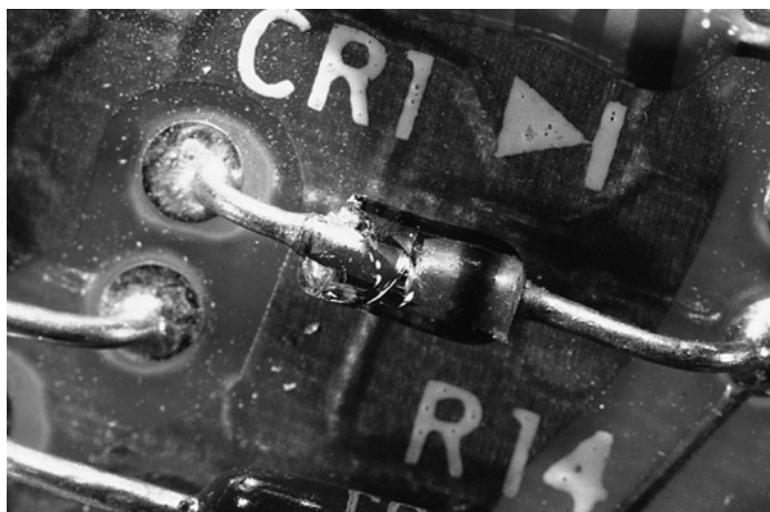
Figure 48 – Damage to axial component with glass body
