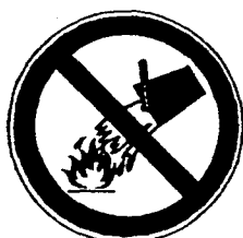
Do not extinguish with water
