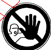
No access for unauthorized persons
