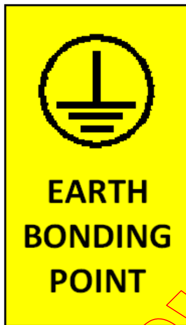
Figure 4 – Example of a label for Type C FIBC designated earth bonding points
