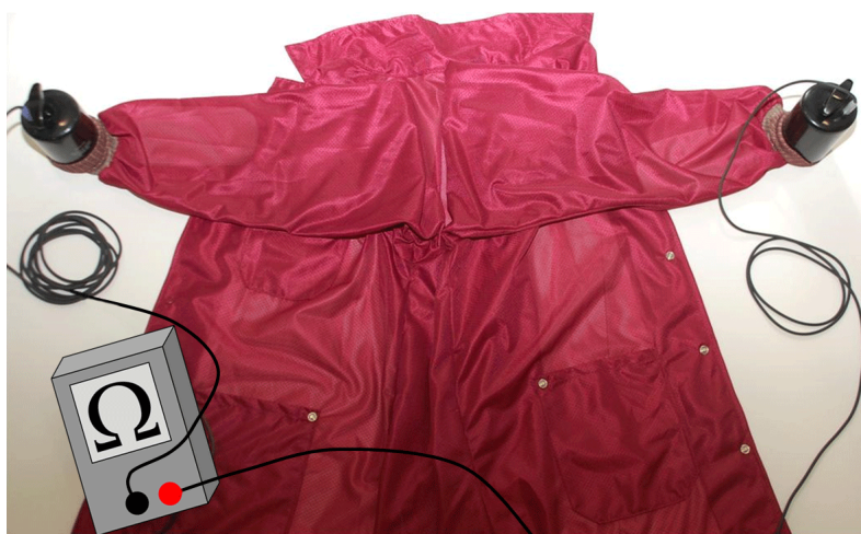
Figure 4 – Test set-up – Resistance point-to-point (cuff-to-cuff procedure with insulative sleeve inserts)
