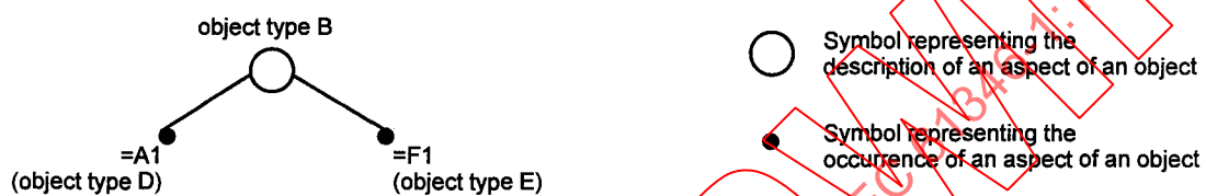
Figure 15 - Function-oriented structure of object type B
