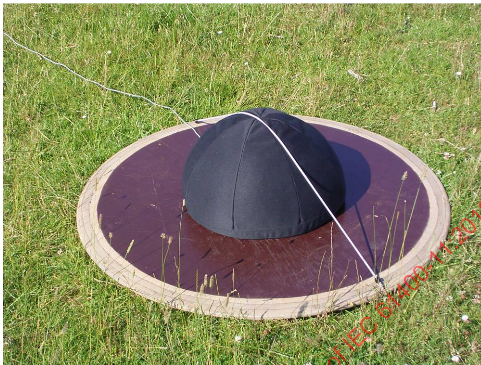
Figure E.2 – Example 2 of secondary wind screen
