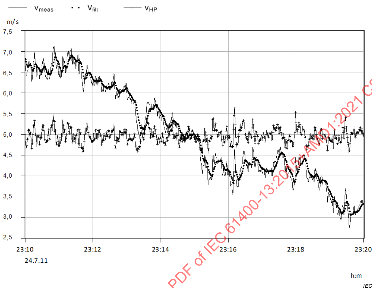
Figure F.1 – Comparison of measured wind speed ( v_{\text{meas}} ), smoothing-filtered wind speed ( v_{\text{filt}} ) and resulting trend-free wind speed ( v_{\text{HP}} )
