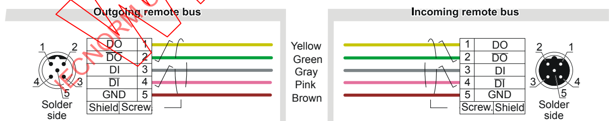
Figure A.5 – M12 circular connector pin assignment
