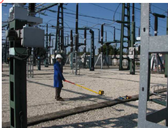
Figure 3 – Electric field measurement using a hand-held stick (photograph RTE)
