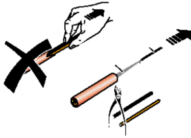
Figure 23 – Do not pull by the individual wires
