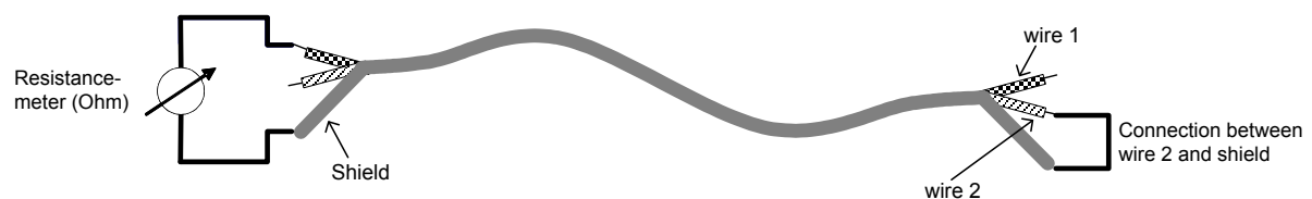
Figure N.4 – Resistance measurement for detecting wire shorts
