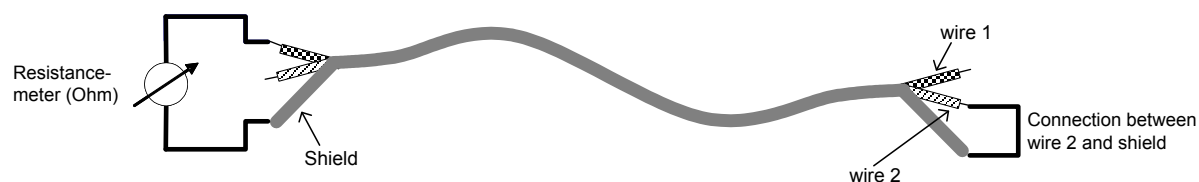
Figure N.4 – Resistance measurement for detecting wire shorts
