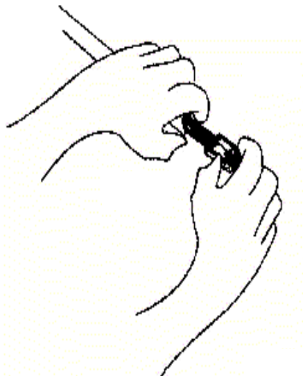
Figure I.4 – Inserting the cable into the connector body
