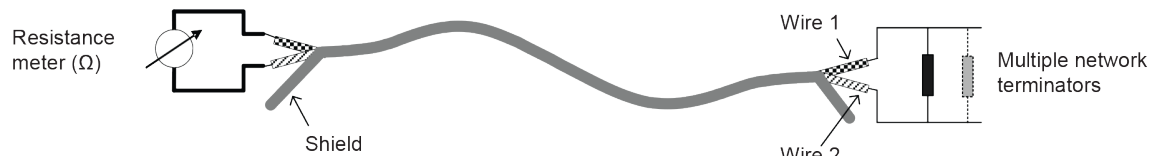
Figure N.5 – Resistance measurement between wire 1 and wire 2
