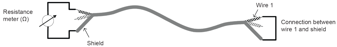
Figure N.2 – Loop resistance measurement wire 1 to shield
