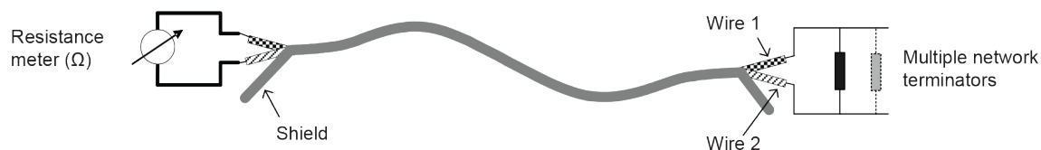
Figure N.5 – Resistance measurement between wire 1 and wire 2
