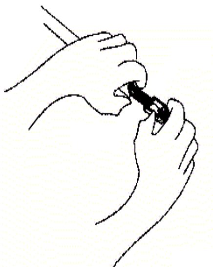
Figure I.4 – Inserting the cable into the connector body
