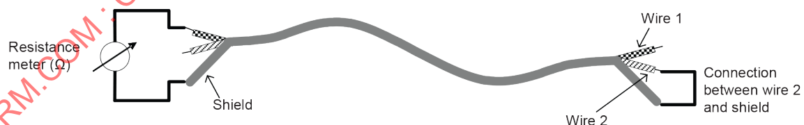
Figure N.4 – Resistance measurement for detecting wire shorts
