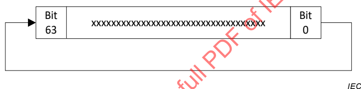
Figure 24 – STA decryption DecoderKey rotation process
