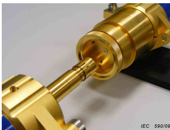
Figure A.7b – Mounted test captivation
