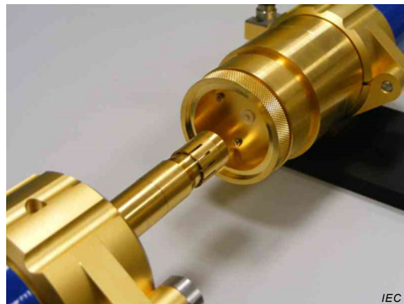
Figure A.7b – Mounted test captivation
