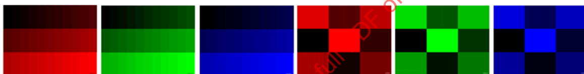
Figure 9 – Test pattern for gamut change of the colour scale
