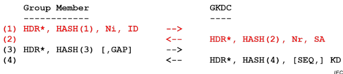
Figure 28 – GROUPKEY-PULL initial SA request exchange
