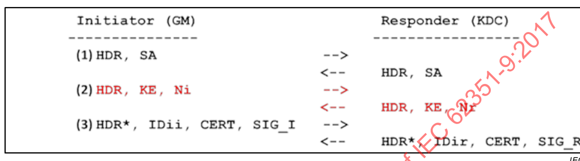
Figure 22 – IKEv1 main mode exchange: key exchange messages
