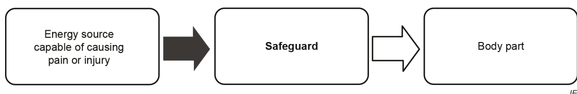
Figure 2 – Three block model for safety
