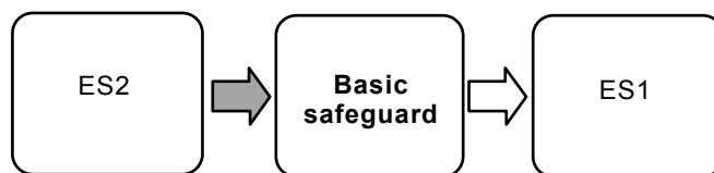
Figure 26 – Model for protection of ES1 against ES2
