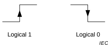
Figure 11 – Bi-phase encoded bits
