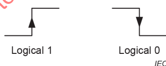
Figure 11 – Bi-phase encoded bits
