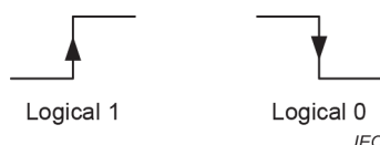
Figure 11 – Bi-phase encoded bits
