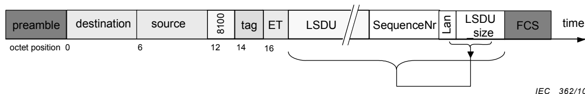
Figure 7 – PRP VLAN-tagged frame extended by an RCT
