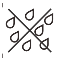
Figure 6 – Lamp not suitable for use under moisture
