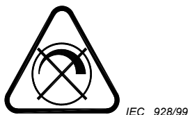
Figure 1 – Dimming not allowed
