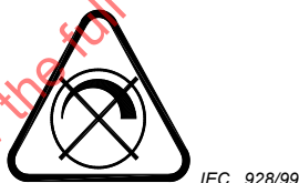
Figure 1 – Dimming not allowed
