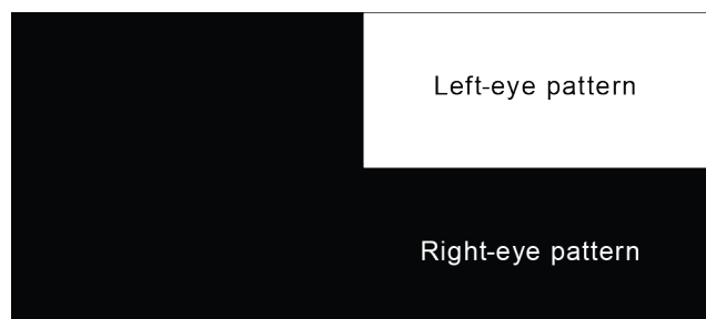
Figure 1 – Example of edge blur test pattern of top/bottom 3D format
