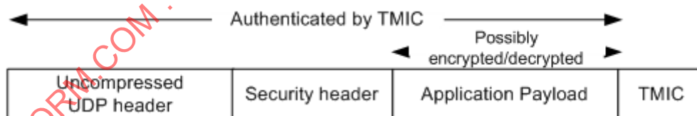
Figure 40 – TPDU structure and protected coverage
