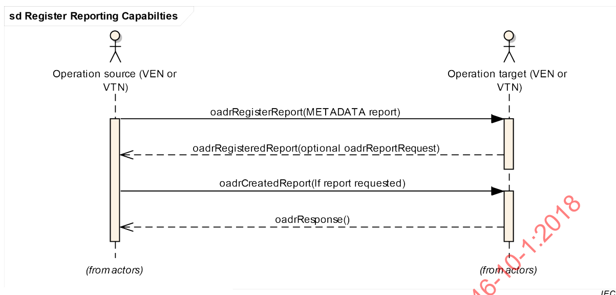
Figure 6 – Interaction diagram: Register reporting capabilities
