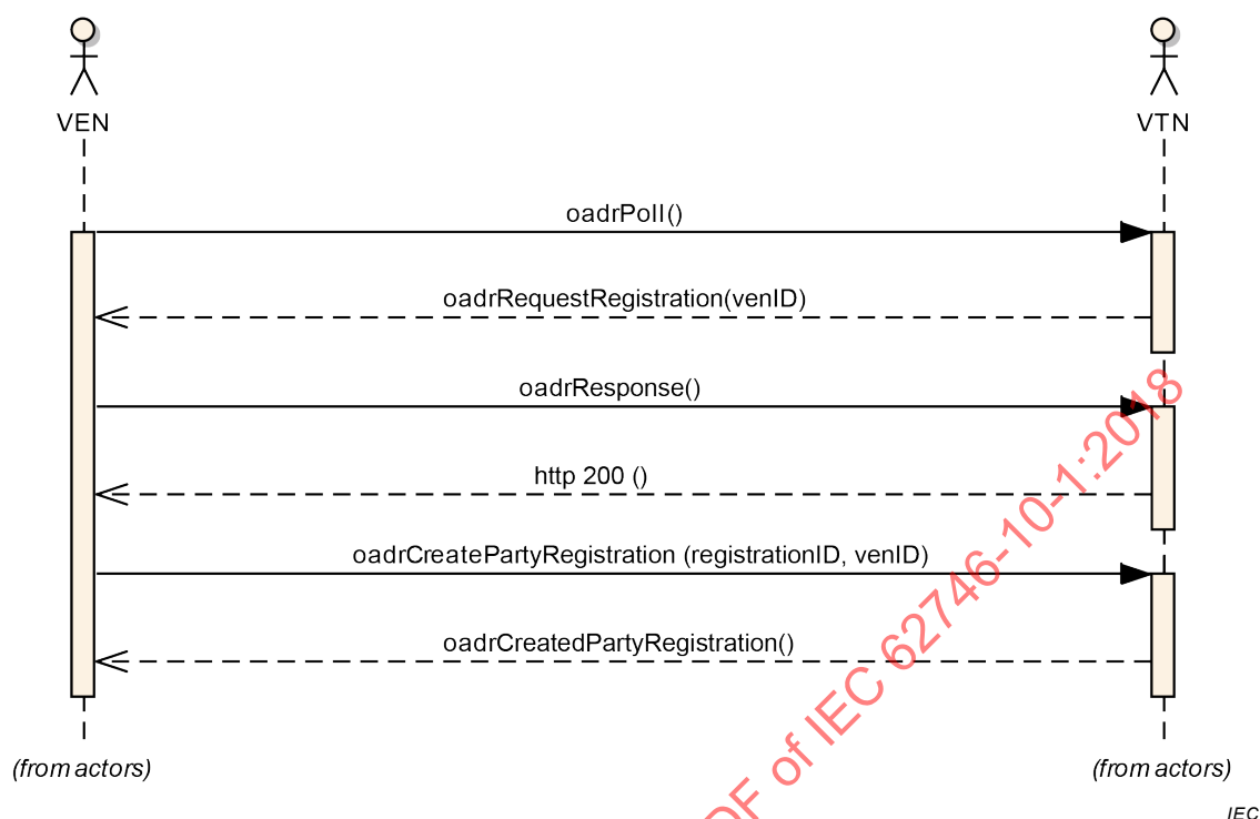
Figure 19 – Interaction diagram: oadrPoll (request reregistration reply)
