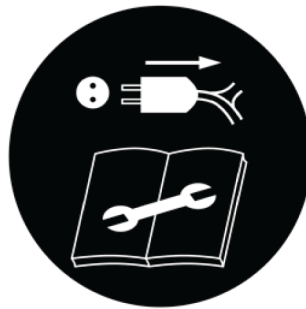
Figure AA.4 – Product safety labels illustrating – "WARNING – Remove plug from mains before maintenance or if the cord is damaged"
