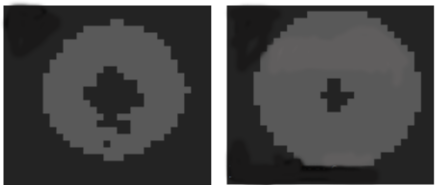
Figure A.2 – Threshold value influence on binary image: on the left, a threshold of 25; on the right, a threshold of 75
