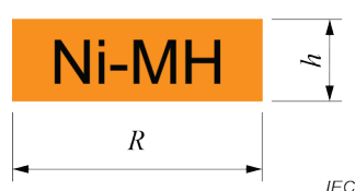
Figure 11 – Size of marking without recycling symbol
