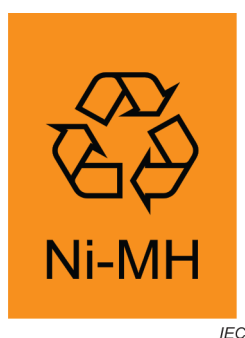
Figure 8 – Example of marking with recycling symbol for nickel metal hydride batteries
