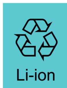
Figure 9 – Example of marking with recycling symbol for lithium ion batteries
