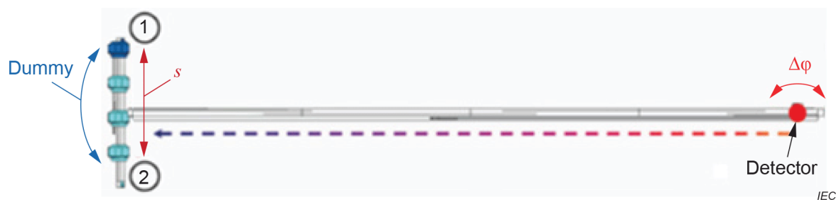
Figure 11 – Test setup for tangential movements (top view)
